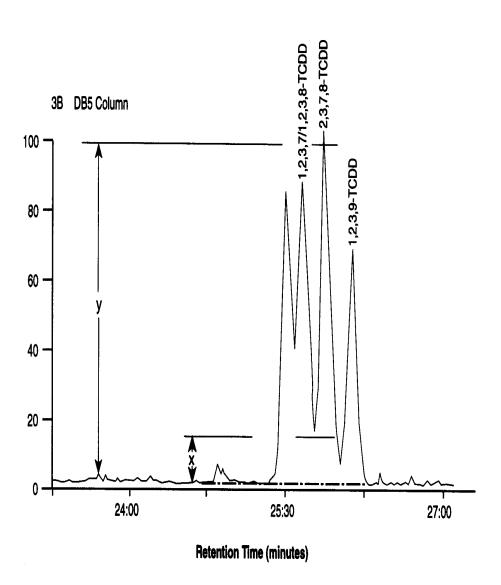
Figure 6. Isomer-Specific Separation of 2,3,7,8-TCDD on DB-5 Column
