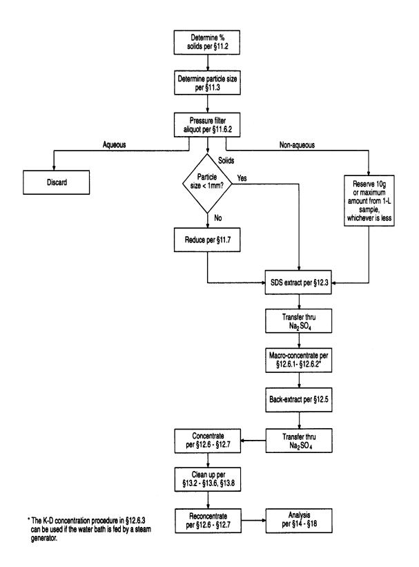
Figure 2. Flow Chart for Analysis of Multi-Phase Samples
