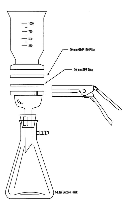
Figure 4. Solid-Phase Extraction Apparatus
