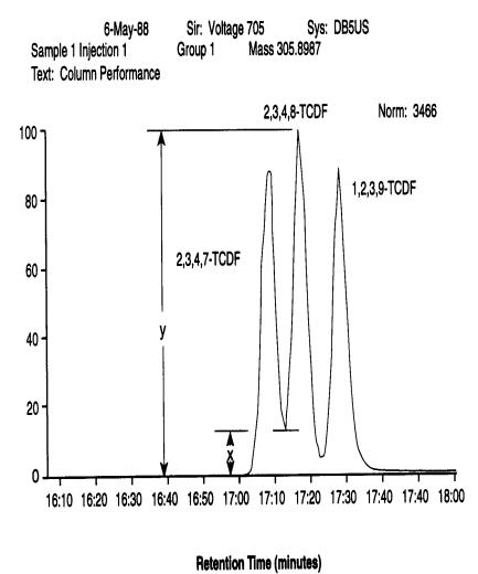
Figure 7. Isomer-Specific Separation of 2,3,7,8-TCDF on DB-5 Column
