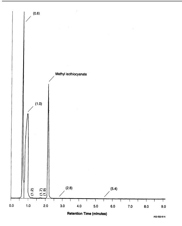
Figure 1. Chromatogram of Methyl Isothiocyanate
