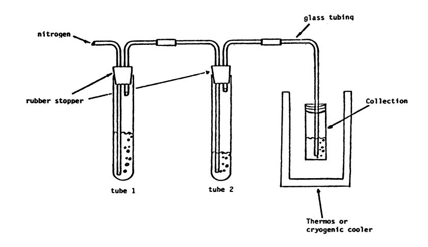
FIGURE 2. DIAZOMETHANE SOLUTION GENERATOR
