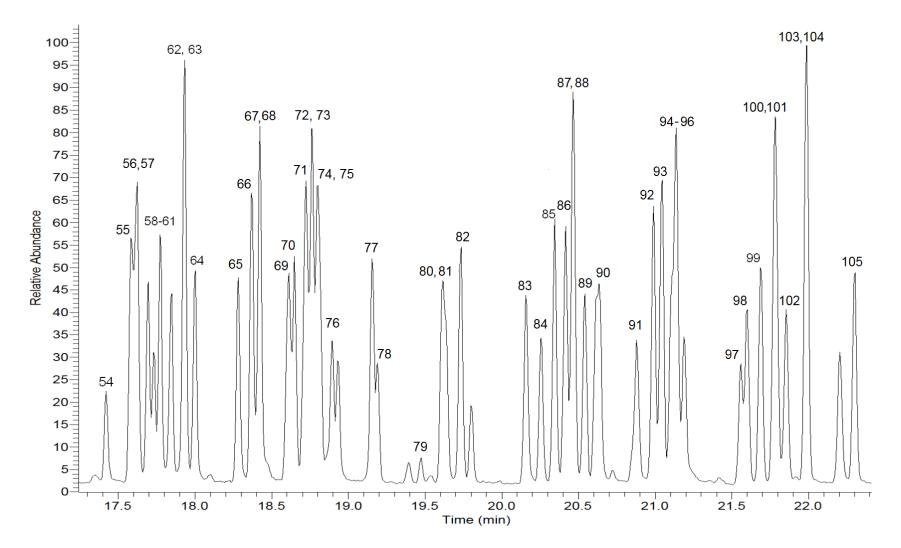
Figure 1d. Example chromatogram of a calibration standard (concentration of 5 ng/µL injected for most analytes). Peak identification numbers correspond to those in Table 1.
