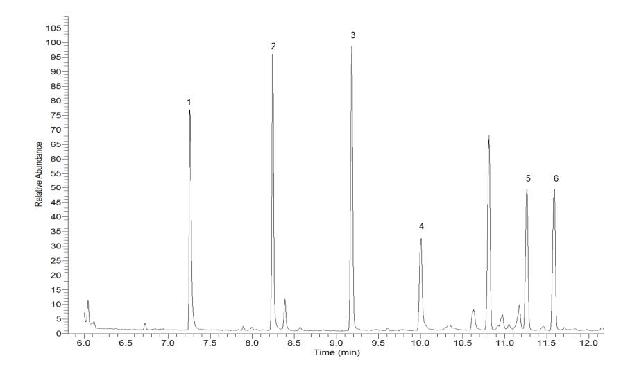
Figure 1b. Example chromatogram of a calibration standard (concentration of 5 ng/ $\mu$ L injected for most analytes). Peak identification numbers correspond to those in Table 1.
