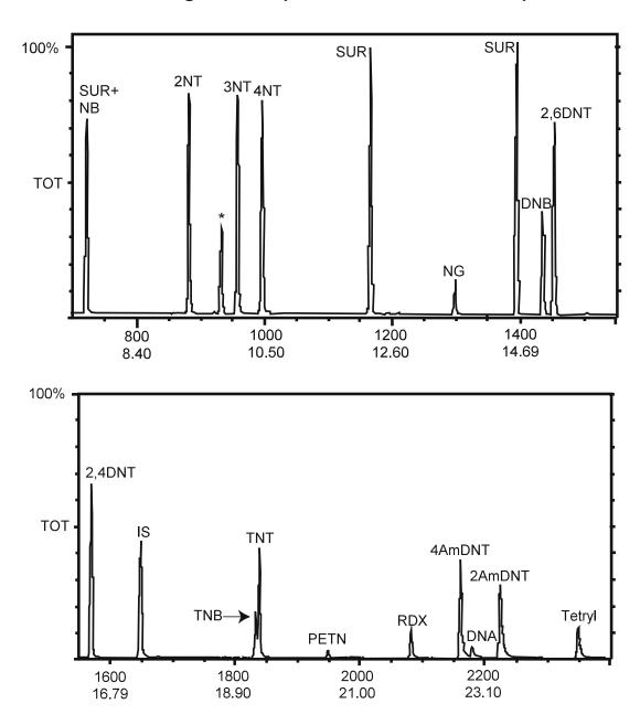
Total ion chromatogram of 16 explosives and related compounds, using a J&W DB5-MS column and the conditions described in Sect. 10.2.2.1; 5ng each analyte, surrogate and internal standard, except DNA which is 1ng. See Table 2 and Sect. 13.2 for compound abbreviations used to label peaks.
