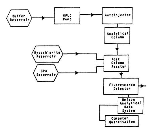
Figure 1. HPLC, Post-Column Reactor System
