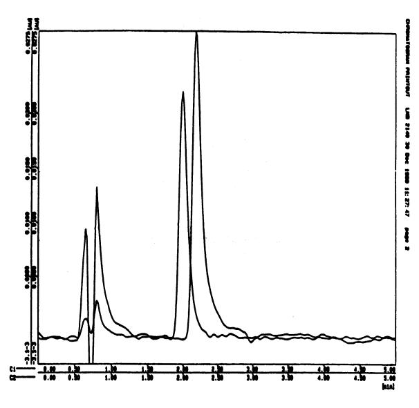
Figure 1. HPLC sample chromatograms of diquat  $(\lambda = 308 \text{ nm})$  and paraquat  $(\lambda = 257 \text{ nm})$ . Retention time of diquat (C = 10 ug/L) is 2.03 min.; retention time of paraquat (C = 11 ug/L) is 2.25 min.
