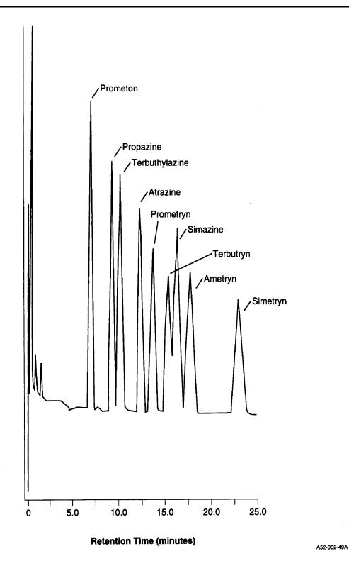
Figure 1. Gas Chromatogram of Triazine Pesticides on Column 1 For Conditions, See Table 1
