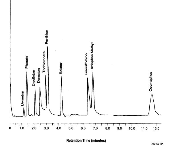
Figure 1. Gas Chromatogram of Organophosphorus Pesticides on Column 1a (for conditions, see Table 1)
