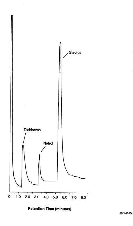
Figure 4. Gas Chromatogram of Organophosphorus Pesticides on Column 3 (for conditions, see Table 1)
