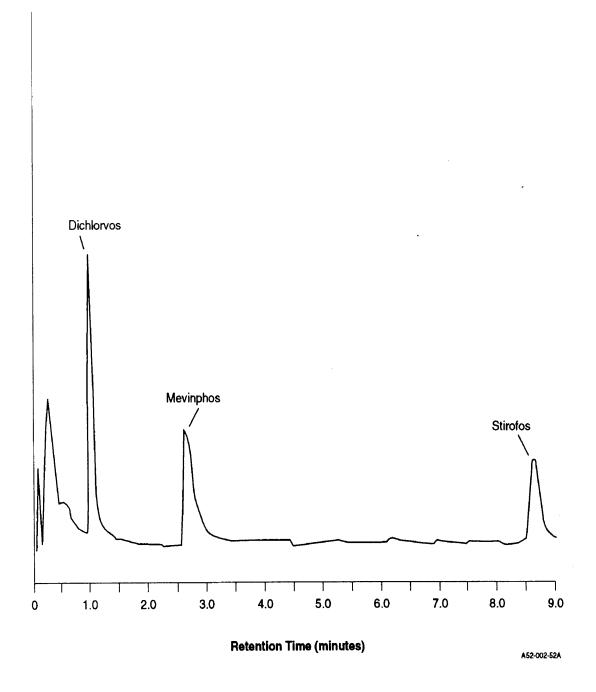
Figure 2. Gas Chromatogram of Organophosphorous Pesticides on Column 1b (for conditions, see Table 1)
