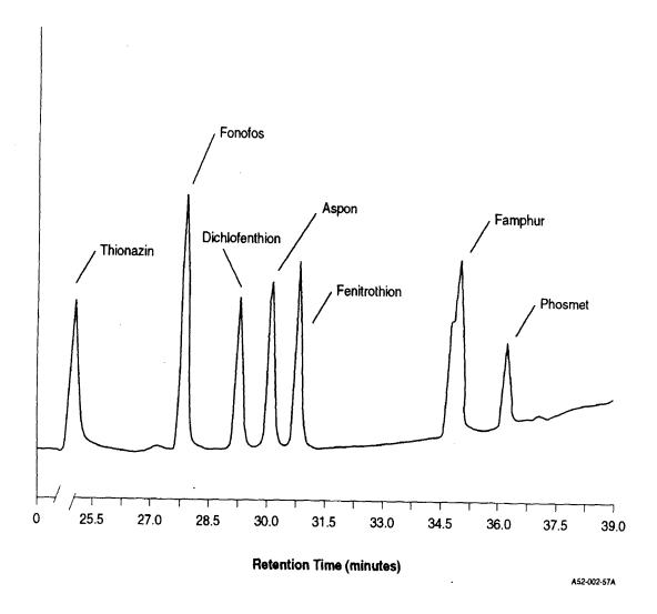
Figure 2. GC-FID Chromatogram of 100 ng Each of Seven Thiophosphates (Column 2)
