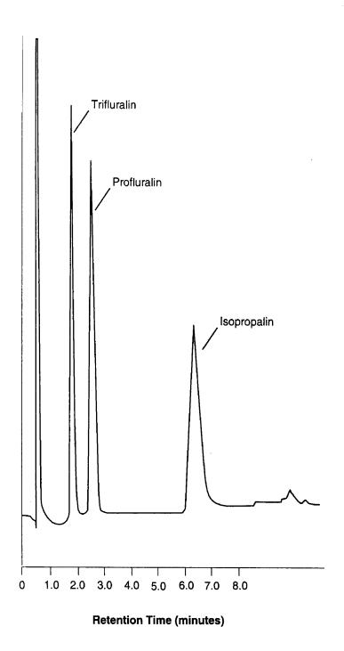
Figure 1. Gas Chromatogram of Dinitroaniline Pesticides on Column 1 (for conditions, see Table 1)
