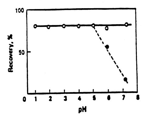
Effect of initial pH on the bromination. Reaction and extraction conditions as in Figure 3. The pH was adjusted to below 3 with concentrated hydrobromic acid, and to 4 - 5 with dilute hydrobromic acid. Reaction at pH 6 was in distilled water. A pH of 7.35 was achieved by careful addition of dilute sodium hydroxide solution. The broken line shows the result obtained by the use of sodium acetate - acetic acid buffer solution.
