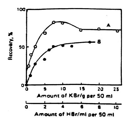
Effect of (A) potassium bromide and (B) hydrobromic acid on the yield of bromination.
