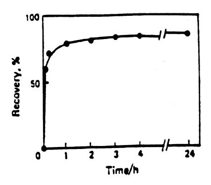
Effect of reaction time on the bromination. Reaction conditions:
