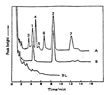
Typical gas chromatograms of the bromination product obtained from aqueous acrylamide monomer solution:
