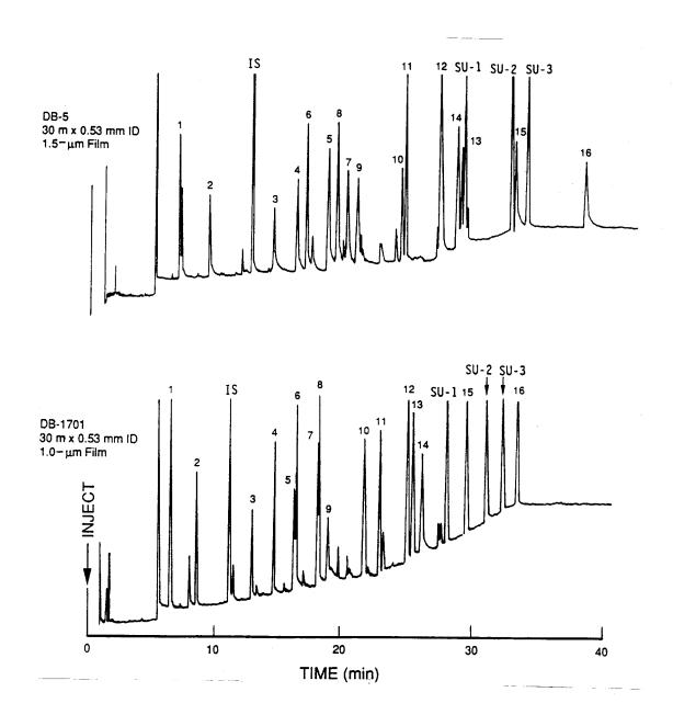
GC/ECD chromatograms of a composite phthalate esters standard (concentration 10 ng/ $\mu$ L per compound) analyzed on a DB-5 and a DB-1701 fused-silica open tubular column. See Table 1 for peak assignments.
