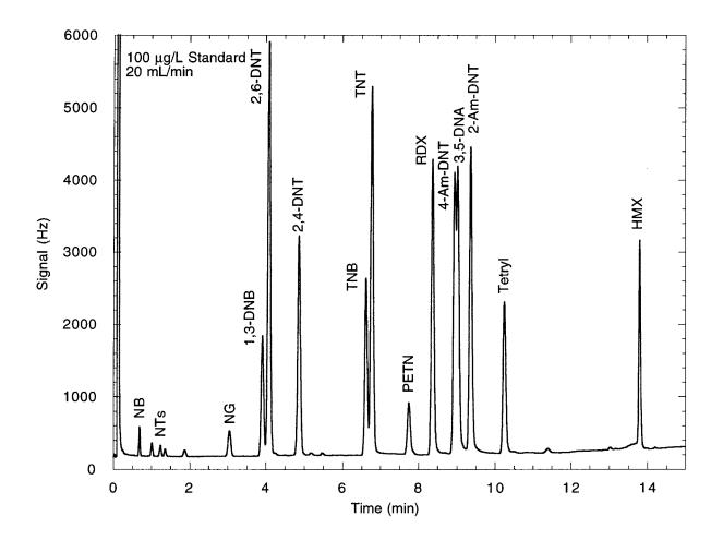
GC operating conditions are listed in Sec. 11.3.3.1. Note the effect of the flow rate on the separation of 4-Am-DNT and 3,5-DNA, as well as on the retention time of HMX.
