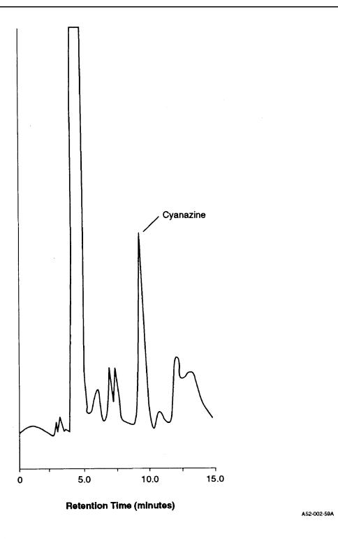
Figure 1. Liquid Chromatogram of Cyanazine in Process Water Extract on Column 1 (for conditions, see Table 1)
