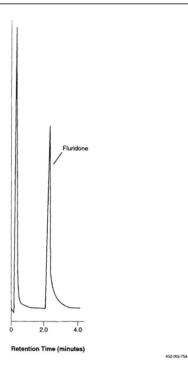
Figure 3. Gas Chromatogram of Fluridone (Column 3)
